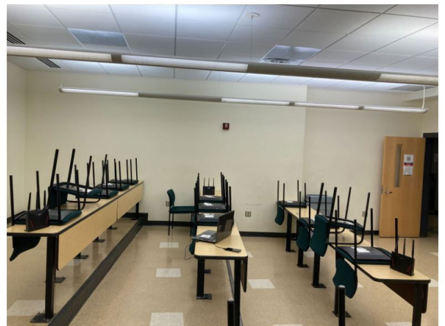
Routers on the far left and far right are communicating with the center router while the phone acts as the sniffer router.
